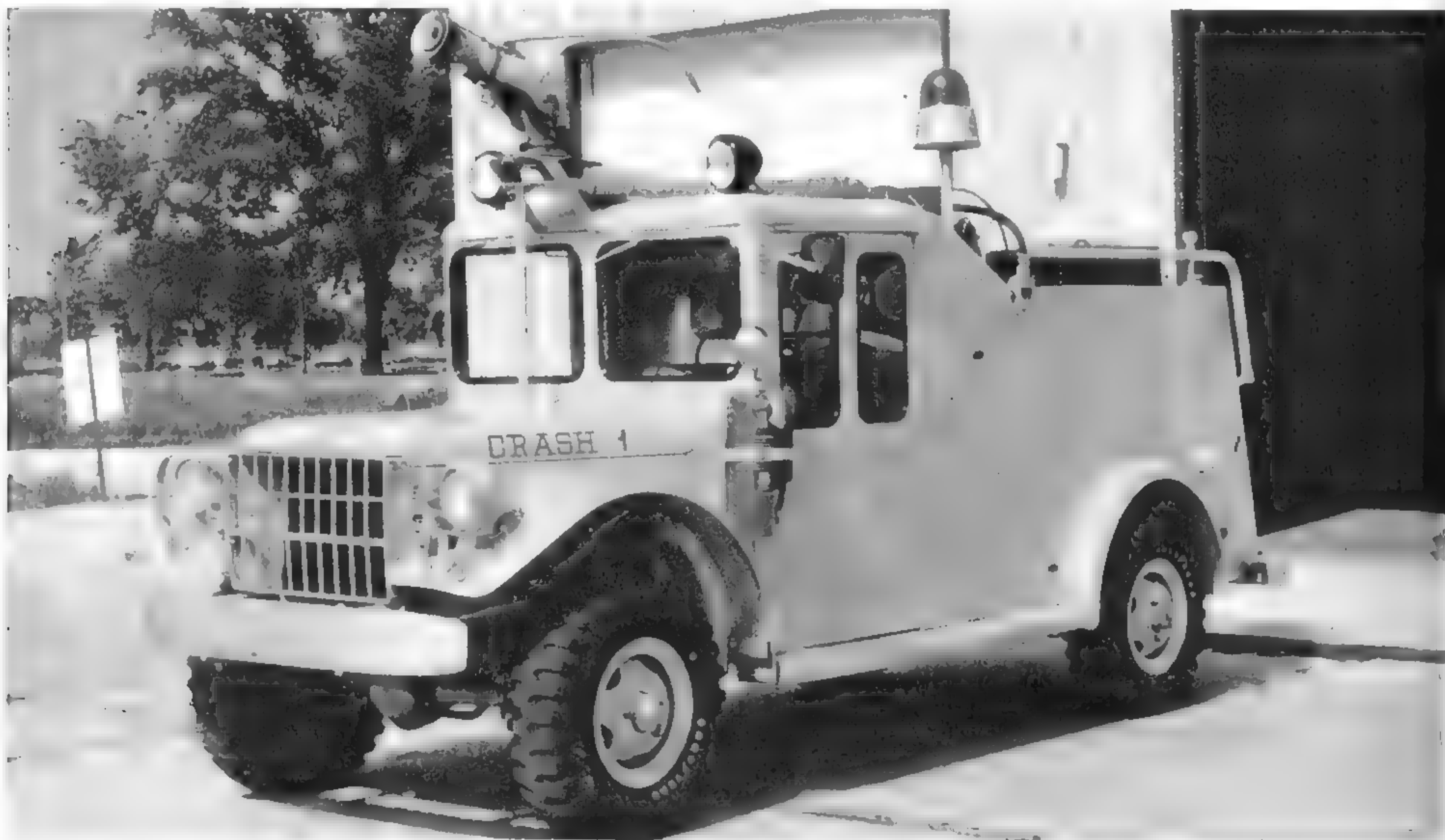
The Navy also had a G-741-based emergency vehicle, the MB-2 Crash Truck. Based on the M56 chassis, the MB-2 had coachwork built by Fred S. Gichner Iron Works of Washington, D.C. Of the reported 200 built, it is not known if any survive intact. This example was photographed in post-Navy service with the West Chicago Fire Protection District. (Photo courtesy of Richard Adelman collection)
